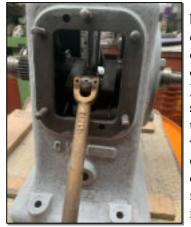
Compressor Connecting Rod Arrangement
